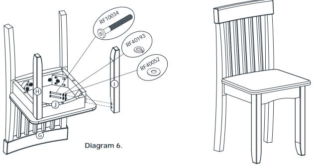
Attach Front Left Leg (H) and Front Right Leg (I) to the Chair Seat Frame (J) by using Screw (RF10034), Spring Washer (RF40193), Washer (RF40052) as per diag. 6.
