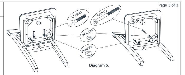
Attach Chair Seat Frame (J) to the Back Rest (G) by using Screw (RF10041), Washer (RF40052), Spring Washer (RF40193) and corner using screw (RF10076), Spring Washer (RF40193), Washer (RF40052) and tighten with Allen Wrench (RF40015)as per diag. 5.
