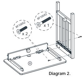
Attach Left Panel (C) into the Desktop (A) and Back Panel (E) using 2 screws (RF10052) and screw (RF10042) as per Diag.2.
