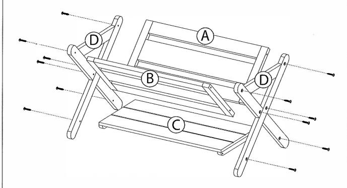
Attach Back Panel (A), Front Panel (B), Bottom Shelf (C) and Side Panel (D) together by using Screws JCA 1/4" x 32mm as per diagram.
